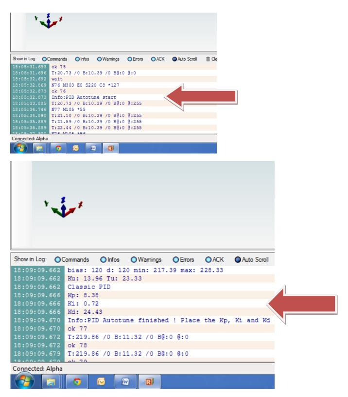
Take note of the (K)P, (K)I and (K)D numbers after the statement 'PID Autotune finished!' is seen in the log
